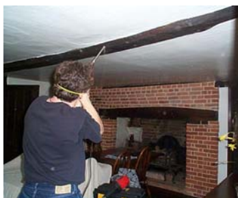
Photo 3: Extraction of a core in progress
